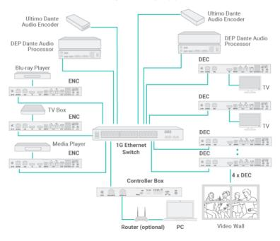
LAN Mode 2 (default): JPEG2000 / Dante AV-A video stream is transmitted through the LAN 1(PoE) port, and Dante audio stream is transmitted through the LAN 2 port.
