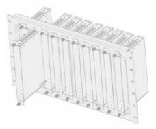
Step 3: Use screws to fix mounting ears on the rack to complete the mounting, as shown in the figure below:
