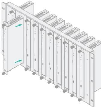
**Step 3:** Use screws to fix mounting ears on the rack to complete the mounting, as shown in the figure below:
