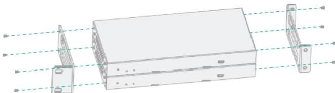
**Step 2:** Fix two 1U rack panels on another two stacked Controllers in the same way, then use screws to fix two 1U rack panels together, as shown in the figure below:
