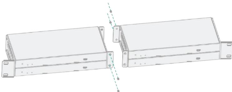
**Step 3:** Fasten screws between two 1U rack panels, so that four Controllers are mounted in a 1U rack, as shown in the figure below:
